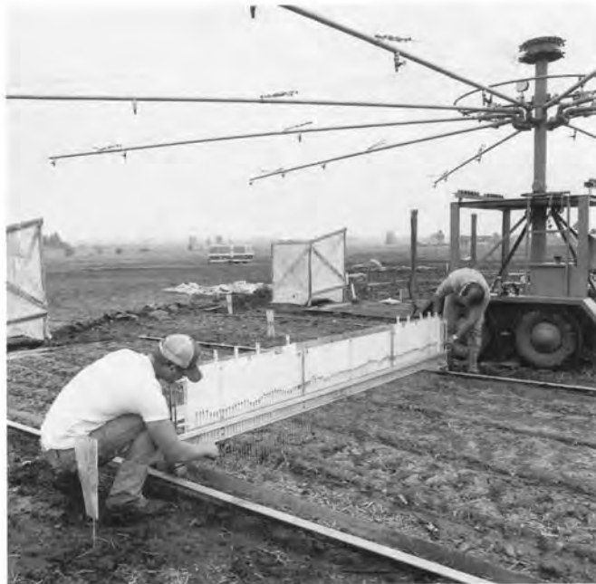
A student measures rill erosion for Kent Mitchell's erosion studies.
