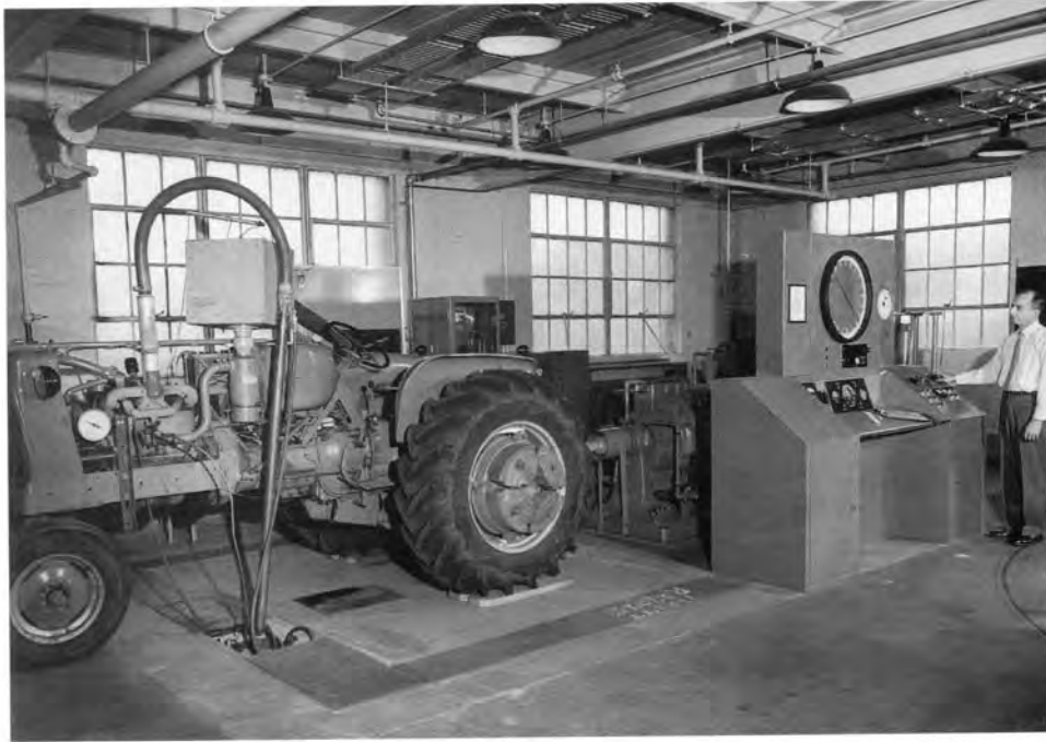
J. A. Weber served as project leader when a 350 horsepower dynamometer to test tractors was added to the tractor maintenance research program in 1961.
