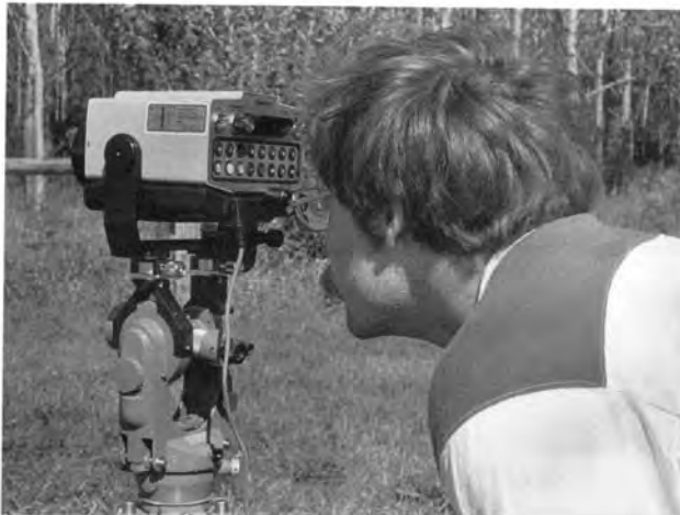
An undergraduate student uses a new electronics distance measuring (EDM) device that replaces the old surveying equipment.
