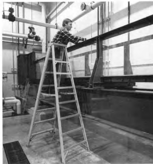
Steve Maddock prepares a large glass-lined flume in the hydraulics laboratory for an erosion control study.
