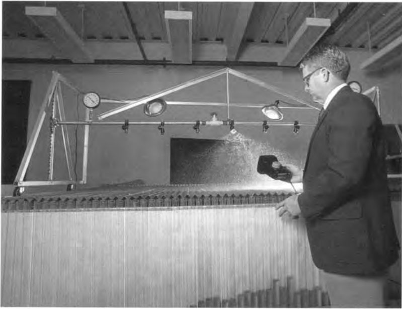
Loren Bode tests spray distribution in the spray laboratory of the new Agricultural Engineering Sciences Building.
