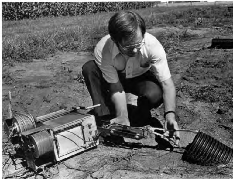
Paul Walker uses the "Illini Mouse" to measure deflection in corrugated plastic drain tubing as part of early studies of proper installation techniques.
