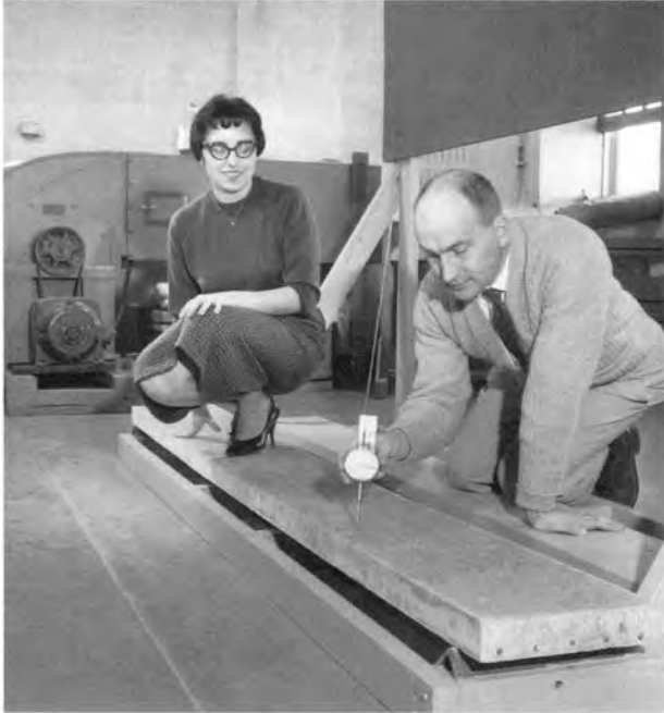
JoAnn Bier assists Don Jedele as he measures precast concrete strength.
