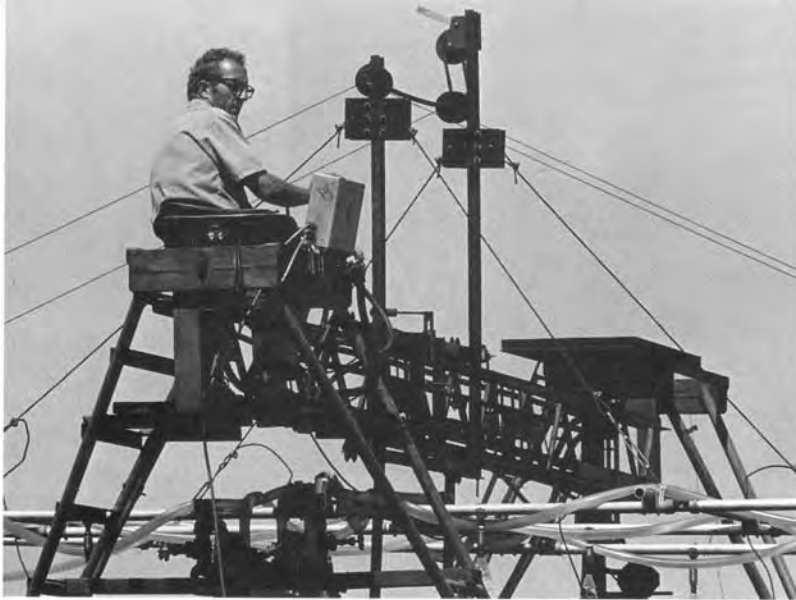
John Siemens atop his "rainmaker" machine for testing soil erosion in the field.
